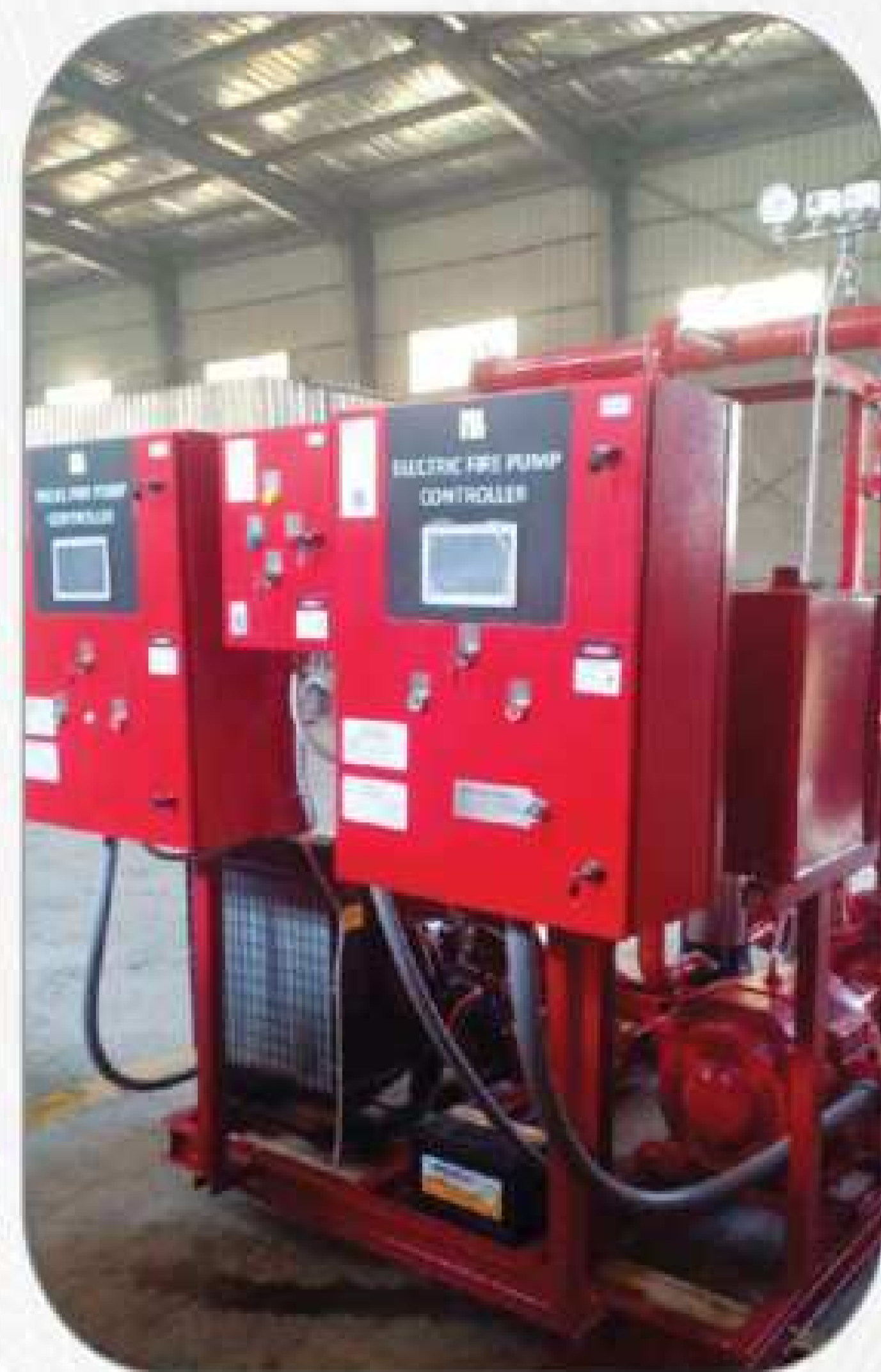
15x fire pump package at the Underground Metro Station – Line 3
